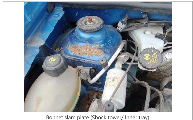
Bonnet slam plate (Shock tower/ Inner tray)
