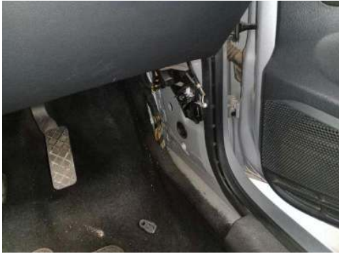
R/F kick panel missing
