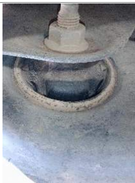
Control Arm Bush(es) Front Axle Right
