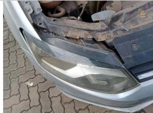
R/F headlight clips broken
