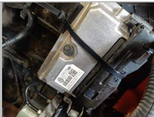
ECU tied with cable ties
