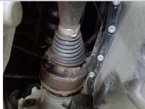
CV Joint(s) Front Right (inner/outer)
