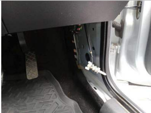
Bonnet release handle missing
