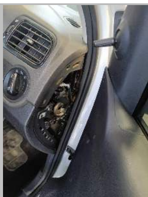
Sider cover missing
