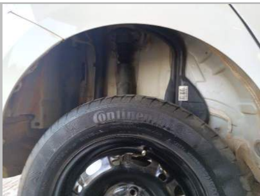
R/R fender liner missing
