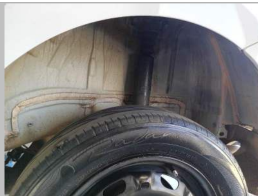
L/R fender liner missing
