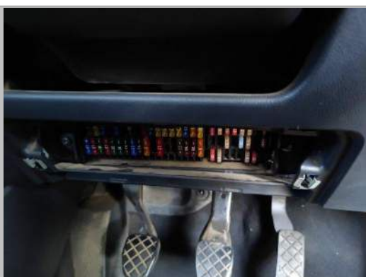
Fuse box and fuses
