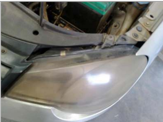
L/F headlight is loose
