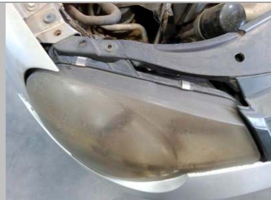
R/F headlight is loose
