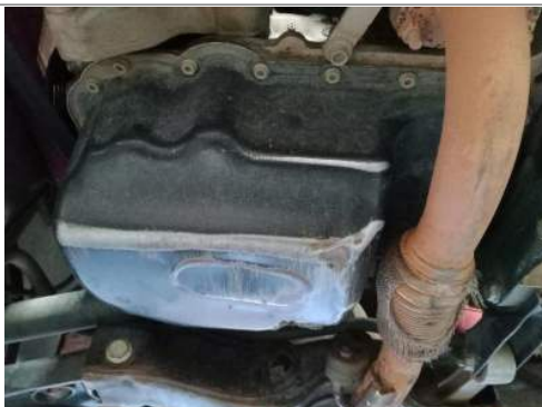
Engine oil sump
