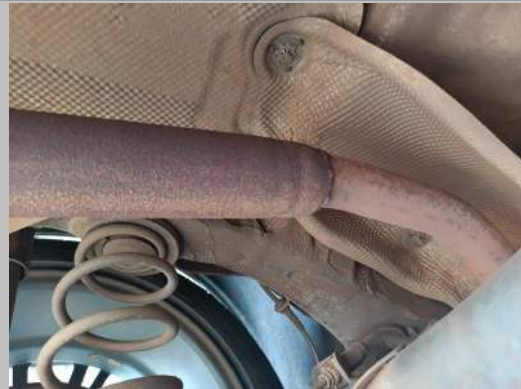
Engine to silencer pipe
