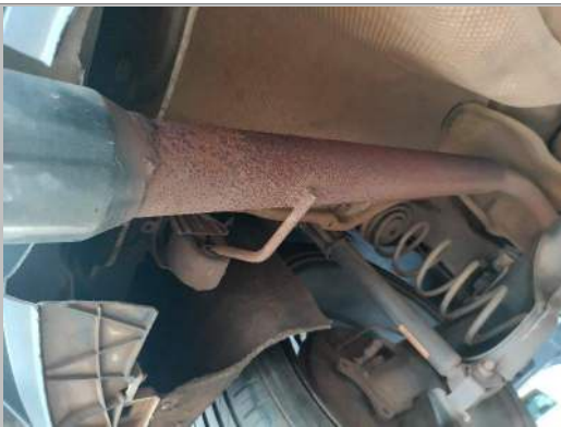
Engine to silencer pipe
