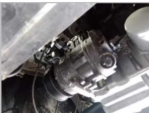
Air conditioner pump
