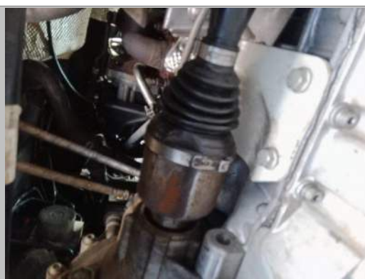
CV Joint(s) Boot(s) Front Right (inner/outer)
