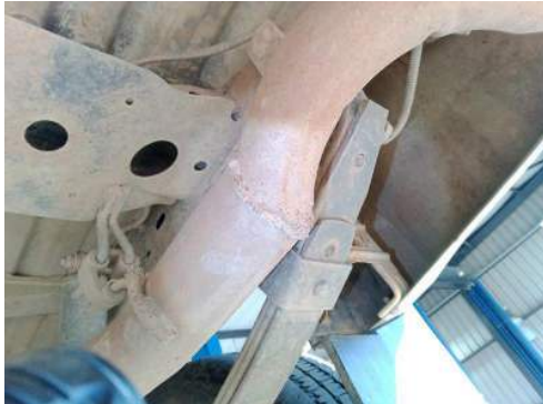
Engine to silencer pipe
