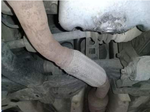
Engine to silencer pipe
