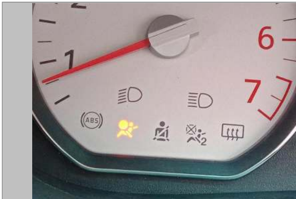
Airbag warning lights illuminated
