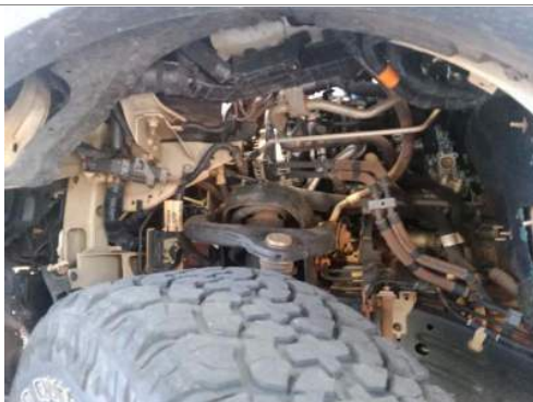
L/F fender liner missing
