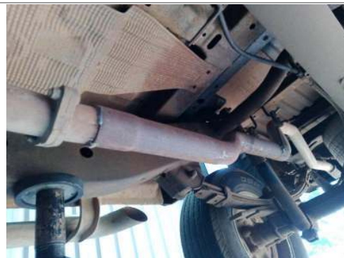
Engine to silencer pipe
