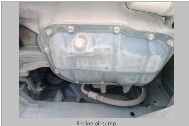
Engine oil sump
