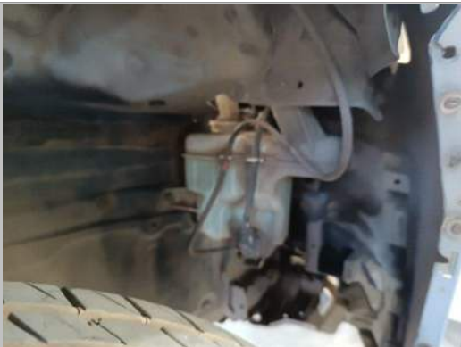
R/F fender liner missing
