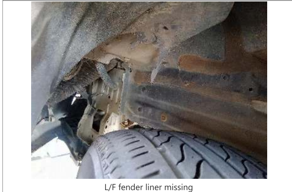
L/F fender liner missing
