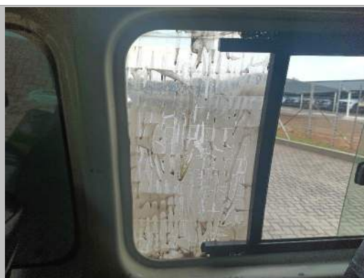
R/R window broken
