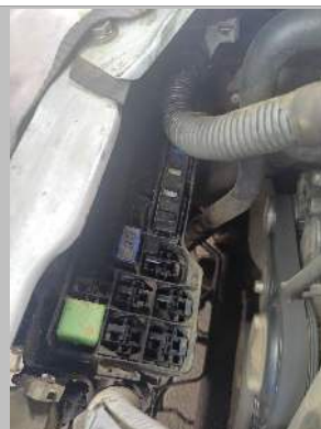
Fuse box and fuses
