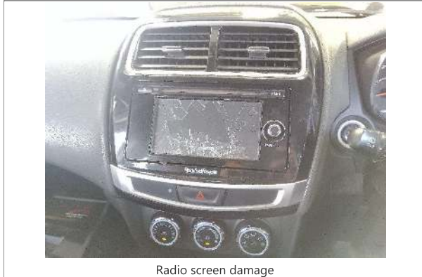
Radio screen damage
