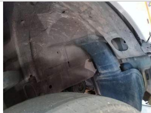
R/F fender liner missing
