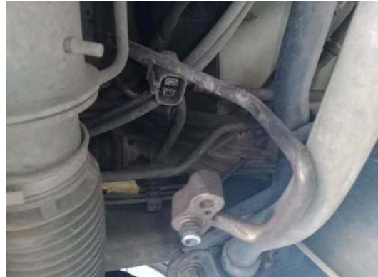
Air conditioner pipes
