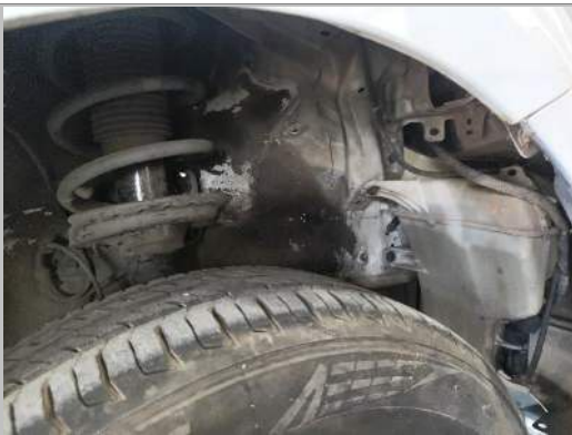
R/F fender liner missing
