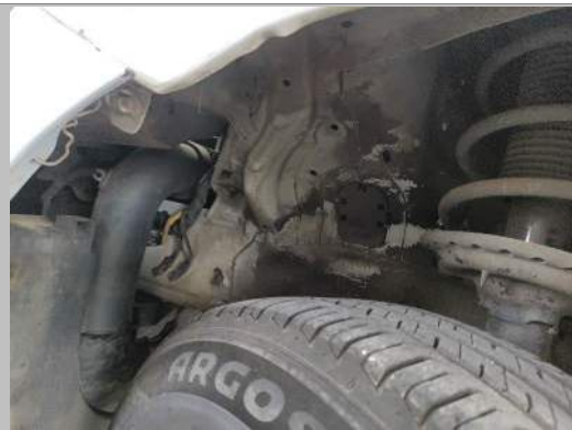
L/F fender liner missing
