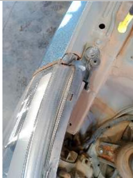
R/F headlight clips broken
