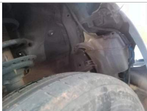
R/F fender liner missing
