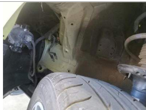
L/F fender liner missing
