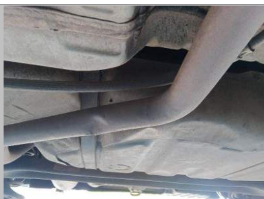
Engine to silencer pipe
