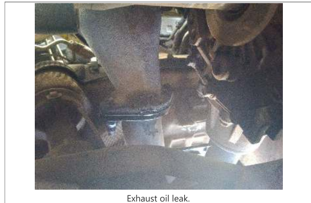
Exhaust oil leak.
