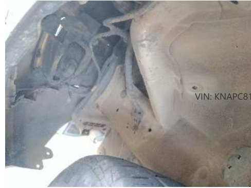
L/F fender liner missing.
