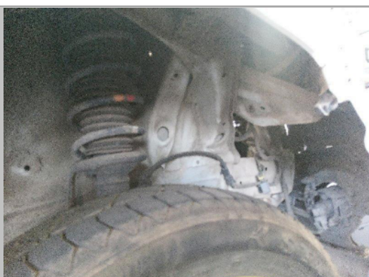
R/F fender liner missing
