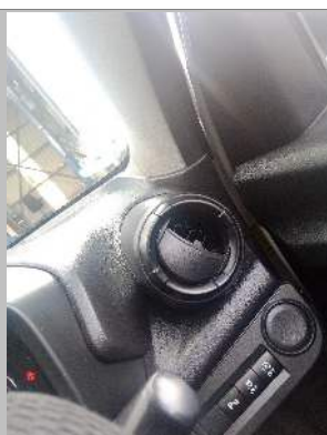
Central Air Vent
