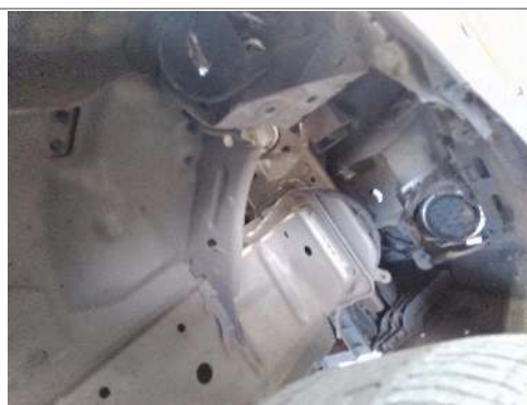
R/F fender liner missing
