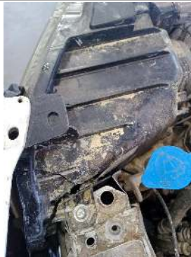
R/F headlight clips broken
