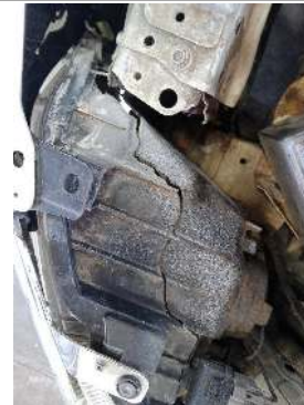
L/F headlight cover broken.
