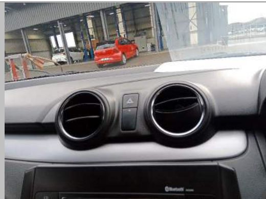
Central Air Vent
