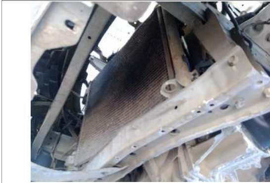
Aircan condenser and radiator.
