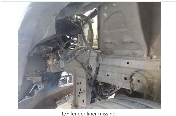
L/F fender liner missing.
