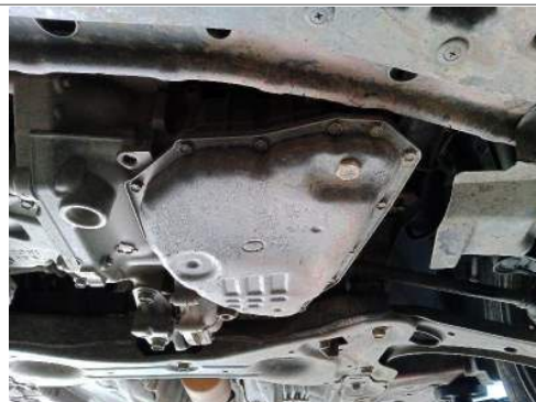
Gearbox oil sump
