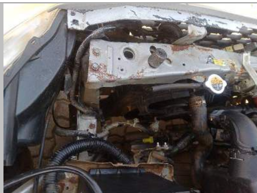
Coolant bottle missing
