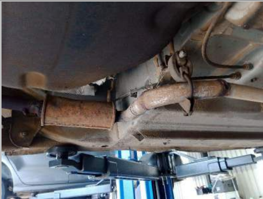
Engine to silencer pipe
