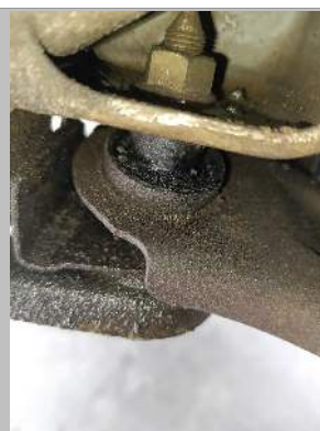
Control Arm Bush(es) Front Axle Right
