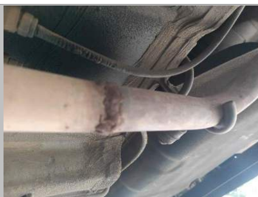
Engine to silencer pipe
