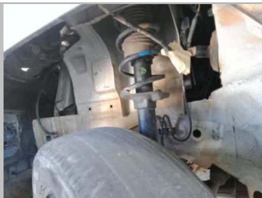
L/F fender liner missing
