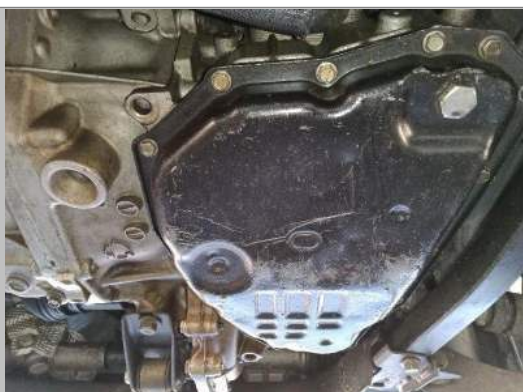
Gearbox oil sump
