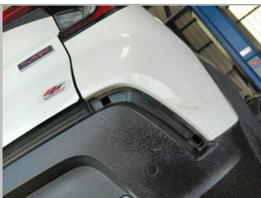
R/R reflector missing
