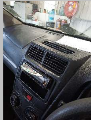
Central Air Vent
