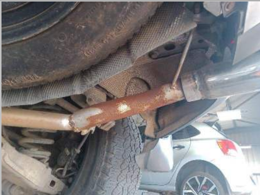
Engine to silencer pipe
