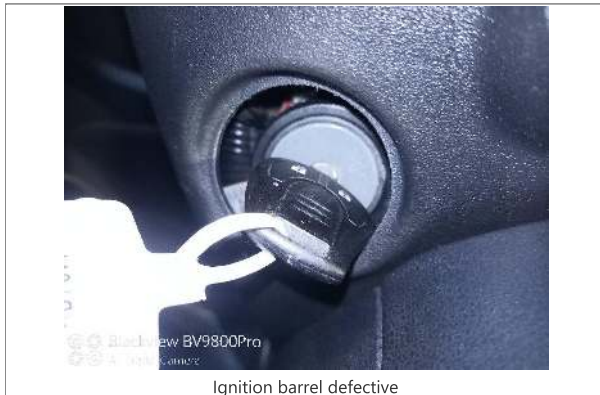
Ignition barrel defective
