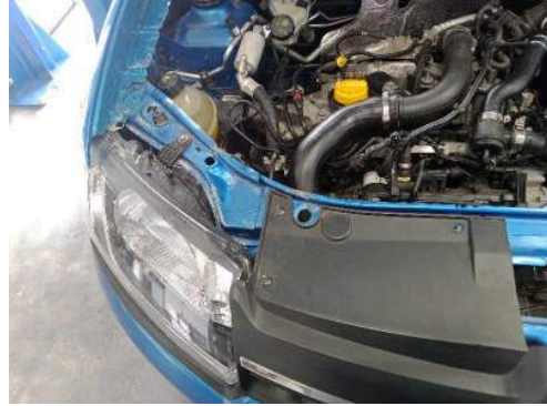
Bonnet slam plate (Shock tower/ Inner tray)
