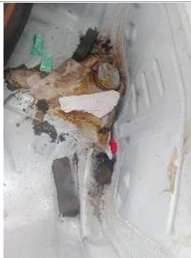
Sparewheel well damage
