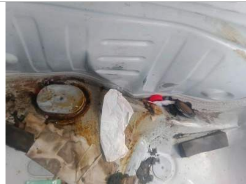
Sparewheel well damage
