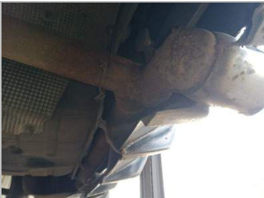
Engine to silencer pipe
