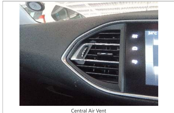
Central Air Vent
