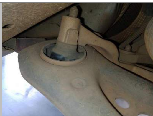
Control Arm Bush(es) Front Axle Right
