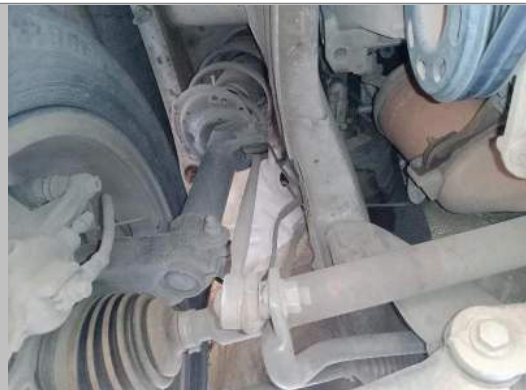
Stabilizer Mounting Front Right
