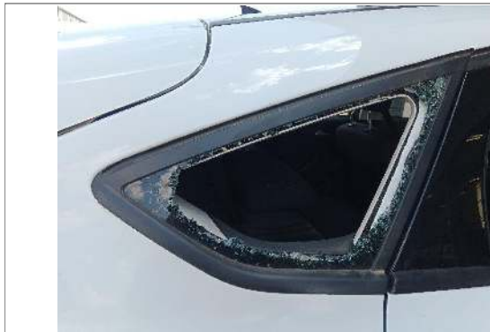
R/R quarter window broken
